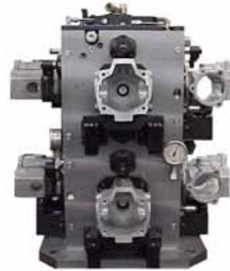
FOUR SIDED TOMBSTONE FIXTURE WITH INTERNAL PLUMBING TO REDUCE CHIP TRAPS
